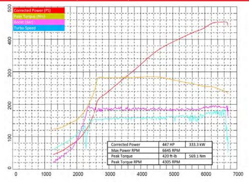
**WARNING:** Maximum allowable turbocharger speed is 186krpm. The use of this product above max turbocharger speed is at the owner's risk, and can result in damage and premature failure. To protect the turbocharger from overspeed when operating, a speed sensor port is machined into the compressor housing for the fitment of speed sensor part numbers 781328-0003 (includes sensor and gauge), and 781328-0004 (includes speed sensor). Speed sensors are sold separately.
