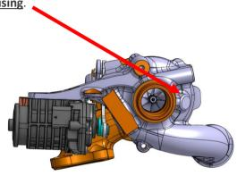
• The correct direct service replacement is as follow: TC PN 870248-5002S replaced by TC PN 887157-5001S as they are using the same e-RCV.
